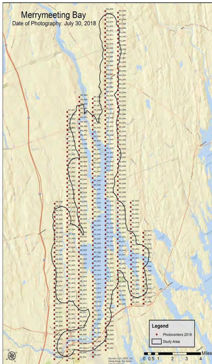
Flight lines and photo stations for stereoscopic imaging
